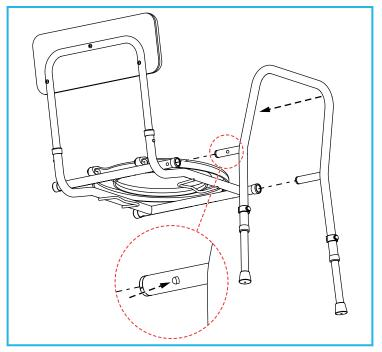
Slide the side assembly into the seat frame assembly.
