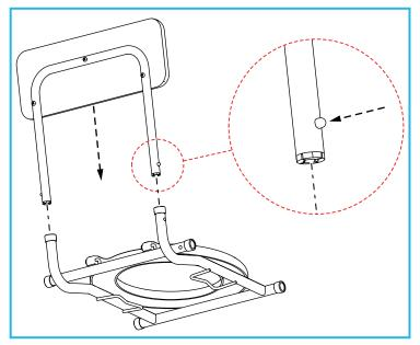
Slide the backrest assembly into the seat frame assembly.
