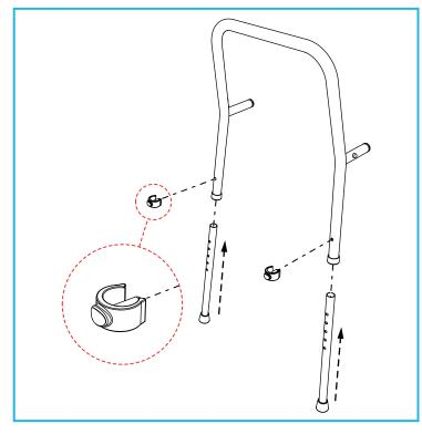
Insert the legs into the side frame and secure with 2 x E-clips.
