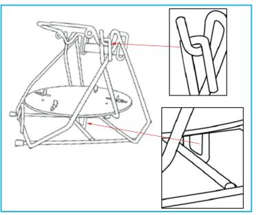
The tilt-plate-stopper must be positioned behind the bar across the base of the frame.
