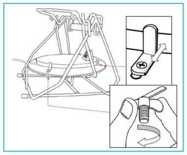
Secure the kettle base onto the tilt plate using the clamps and wing-nuts provided.
