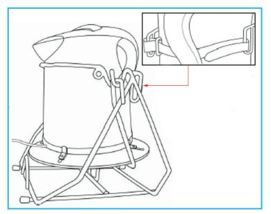
Place the kettle onto the tipper and fasten in position by attaching the Velcro strap.
