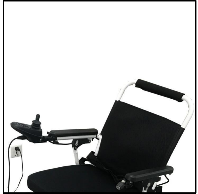
Figure 12. Battery Charging using the Off-board Charger
