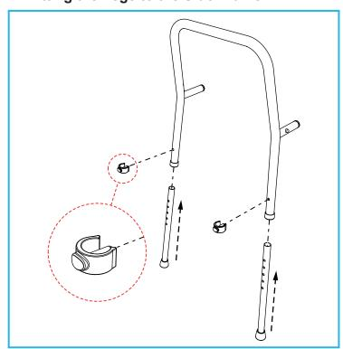
Insert the legs into the side frame and secure with 2 x E-clips.
