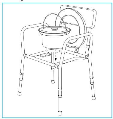
Place the commode pan onto the retainers, on either side of the seat frame.
