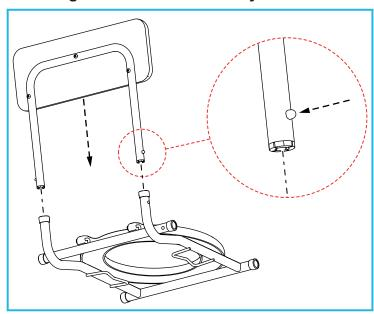
Slide the backrest assembly into the seat frame assembly.
