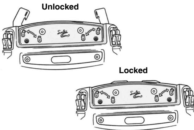
**PLEASE NOTE:** The platform flaps may become stiff following long periods of storage, this can be cured by fully opening and then closing each flap, repeating as necessary until each flap moves easily.
