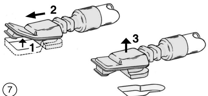
To unfasten the plastic lugs in order to remove the backrest and platform pad:-
