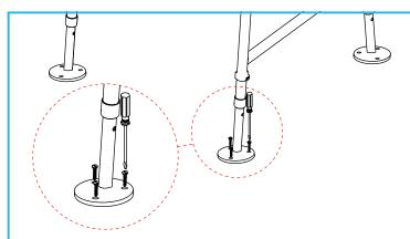
1. Using an appropriate tool for the chosen fixings, secure the floor fixing kit feet to the floor.
