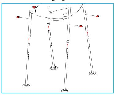
1. Insert the floor fixing kit legs into the toilet frame.
