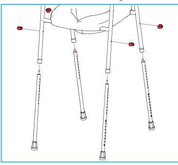
1. Remove the 4 x E-clips, then remove the toilet frame leg extensions.
