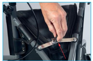
Pull the crossbar handle towards you to unlock the frame, then push the handles together to fold the rollator.
