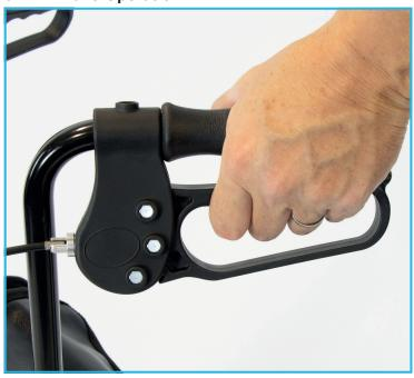
To slow down or stop the rollator, pull both brake handles up.
