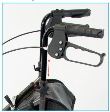
Undo and remove the hand wheel by turning anticlockwise.
