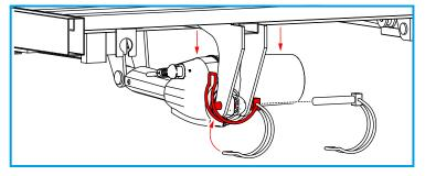
2. Lower the actuator into place, then line up the holes and replace the pin-clip.
