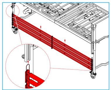
3. Insert the plastic side rail carriages into the side rail channels, taking care not to snag the wires.
