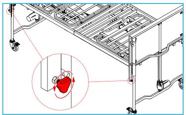
2. Undo the 2 x locking screws on one side of the bed.
