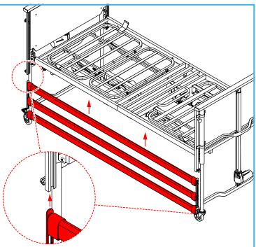
3. Insert the plastic side rail carriages into the side rail channels, taking care not to snag the looped wires.
