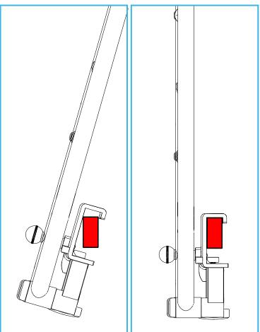
3. Tilt the side rail forward and clip over the bed platform, then slide the bottom fixing under the bed platform by straightening up the side rail.
