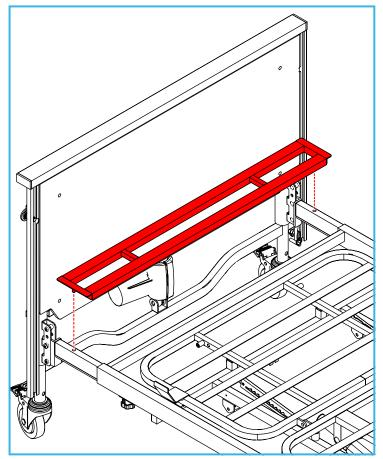
3. Fit the mattress platform extension plate in the position shown.
