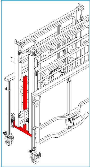
12. Slot the mattress platform connectors on to the transport bracket.
