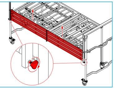
4. While holding the side rail assembly in place, tighten the locking screws at both ends of the bed.
