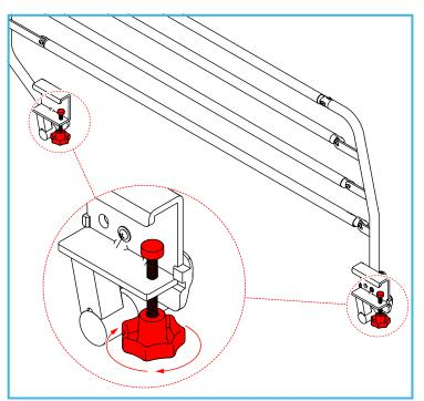
1. Loosen the side rail hand-wheels all the way.
