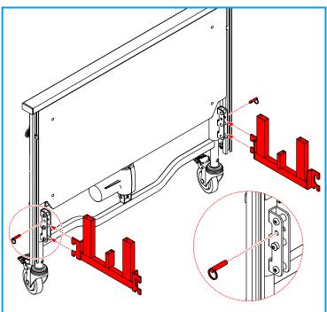
3. Hook the transport brackets onto the foot end panel brackets (lower pins) and secure with the retaining pins on both sides.
