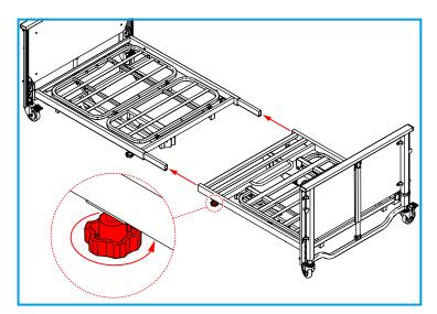
5. Loosen the hand-wheels fully on the head end mattress platform by turning them anticlockwise on both sides.
