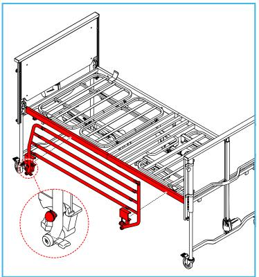
2. Position the side rails so the locking lever knob is always at the foot end of the bed.
