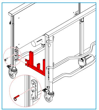
4. Hook the transport brackets onto the head end panel brackets (lower pins) and secure with the retaining pins on both sides.
