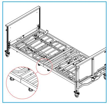
6. Slot the head end mattress platform onto the platform connectors until it is flush with the foot end mattress platform.
