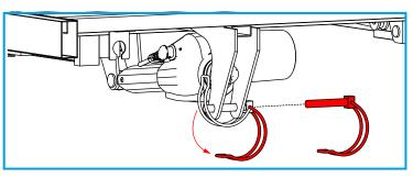
1. While supporting the actuator, remove the pinclip.
