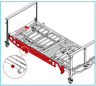
Lift the top rail of the side rail assembly all the way up until the sprung knob clicks into place.
