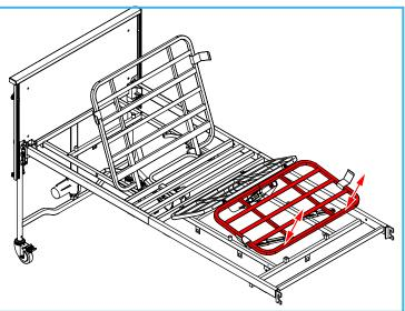
Manually lift the end of the calf section to the highest point (this releases the catch) then lower.
