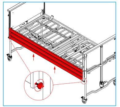
4. While holding the side rail assembly in place, tighten the locking screws at both ends of the bed.
