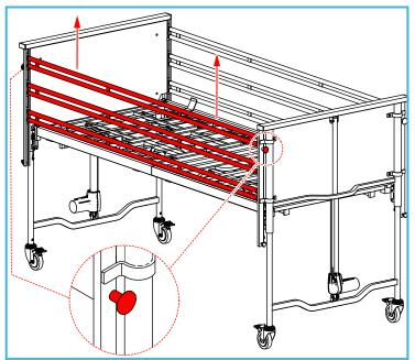
Lift the top rail of the side rail assembly all the way up until it clicks past the spring-plungers at both ends of the bed.
