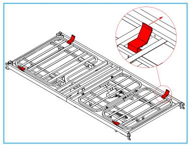
Clip the plastic mattress retainers to the back rest and leg-rest frames in the positions shown.
