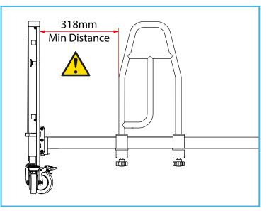
The grab handle must be installed before fitting the side rails.
