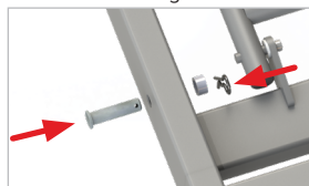
8.2.5 Clevis pin, spacer, and R clip fitting
