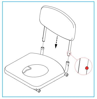
Slide the backrest assembly into the seat frame assembly.
