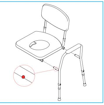
Slide the side assembly into the seat frame assembly.
