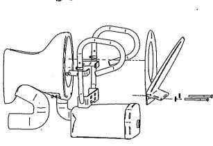
2. Hand-tighten side bolts so that rubber caps firmly contact side of toilet bowl
