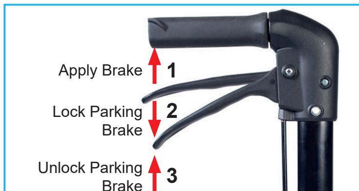
Figure 9: Operating the Brakes
