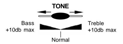
**Note:** When the tone (treble), earpiece volume and sending levels are set to the maximum, whistling may occur. Then the sending level settings should be decreased with the switch
