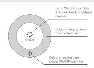
By holding on to the 'Colour changing base - power ON/OFF touch key' - ① for 3 seconds, the base will then begin to change colour automatically (cycling through the colour spectrum)
