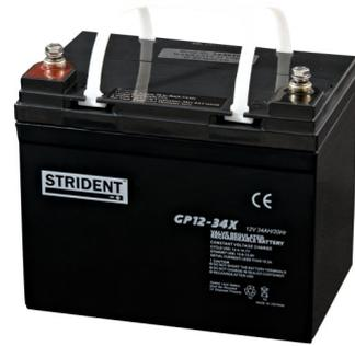
The rechargeable batteries are lead-lead dioxide systems. The dilute sulfuric acid electrolyte is absorbed by separators and plates and thus immobilized. Should the battery be accidentally overcharged producing hydrogen and oxygen, special one-way valves allow the gases to escape thus avoiding excessive pressure build-up. Otherwise, the battery is completely sealed and is, therefore maintenance-free and leak proof. Batteries should be used in an upright position only.
