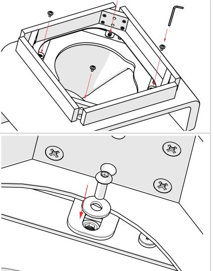
Use the Hexagon Tool to attach the Wooden Base Frame Assembly to the chair. Use the four Socket Head Screws and large Plain Washers.
