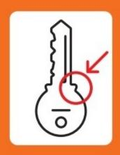
If your key looks like this (with a shoulder) at **Step 3**, make sure key is FULLY inserted while pressing Lockpal into place.
