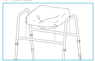
Remove the seat from the bag and snap into place on the centre bars of the frame.
