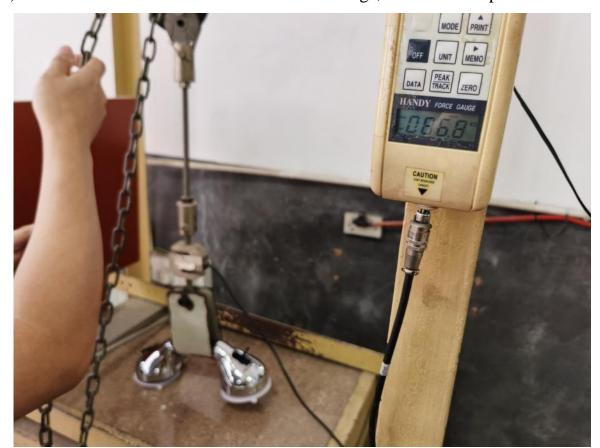
Test summary: The max suction power of this product is around  $154\ lbs$  /  $70\ kgs$ , the product will fall off or broken if the tensile force over  $154\ lbs$  /  $70\ kgs$ .
