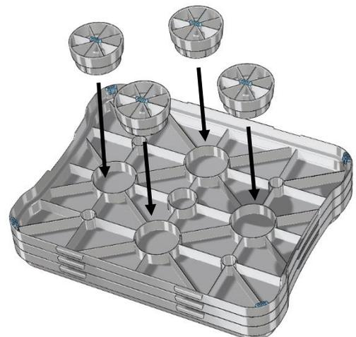
Figure 2 – Fitting the Support Pillars
