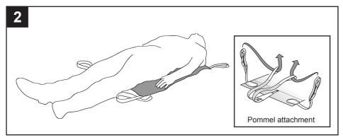
Carefully roll the patient onto the sling far enough so that the sling can be fully unrolled and the patient laid flat and central on the sling. Pass each leg strap through the corresponding loop on the pommel according to the illustration above.
