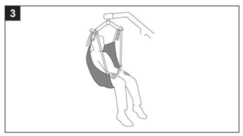
Move the lift into position above the patient. Attach the side suspenders (if used), keeping them away from the patients face. Attach the shoulder straps and leg loops to the respective front and rear hooks on the spreader bar, ensuring the same coloured loops are used on each side.
