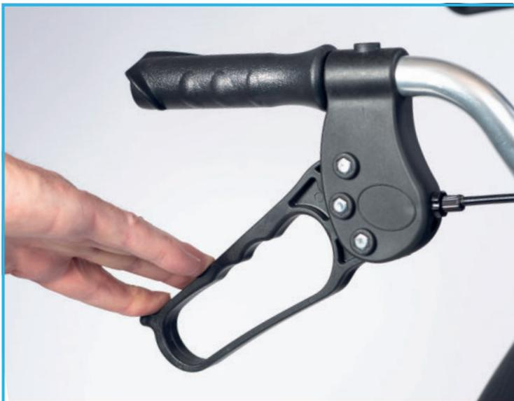
To apply the parking brake, push the brake handles down until they lock into place.
