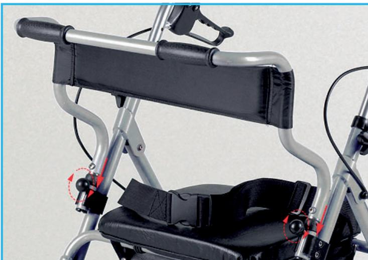
Position the backrest (2) bar so that the push handle is facing away from the seat, then insert into the push handle location sockets (4) and secure using the 2 x hand-wheels provided.
