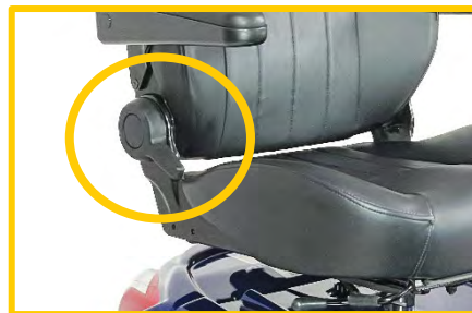
Figure 4 – Pull black handle to adjust the backrest
