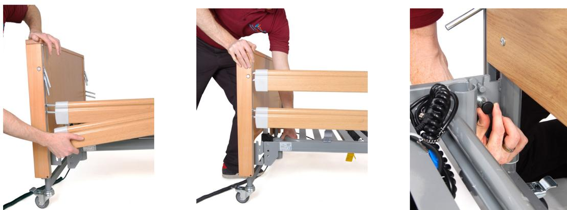
With the side guards slotted into place, the end panel can be pushed back up to the mattress base and secured with the mounting lug. Repeat this procedure on the other side of the bed with the remaining two side guards and fix the two spring-loaded catches securely to the mattress base.
