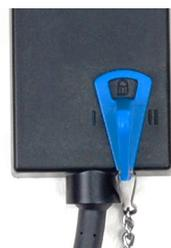
The switching positions I and II are testing settings, used to check the safety during the annual inspection or after repair work, or each time the bed is put into service again.
