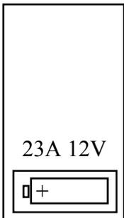
Remove battery cover by sliding down. Insert battery as shown. Replace battery cover. Press blue button to transmit message. Blue LED will light to confirm transmission. Red LED indicates low battery.
