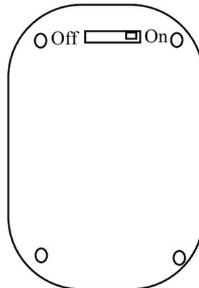
A battery will be pre-installed. Slide the switch to on position. Press blue button to send message. To replace battery, remove four screws then lift away bottom section of box. Replace battery with a good quality Alkaline 9 Volt battery. Replace screws.
