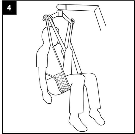
Raise the hoist to the required height. When reseatng the client, apply light pressure on the client's thigh(s) to ensure good posture is maintained.
