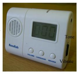
The pager can operate in vibrate or sound mode. To use the pager in sound only mode, slide the switch to the double note mark. For vibration only slide the switch down towards the double note with two lines.
