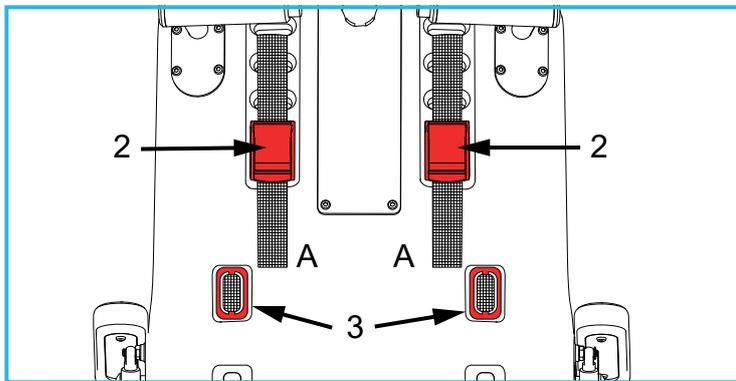
2. Feed the upper straps (A) down through the cam-locks (2), then lock the cam-locks closed.
