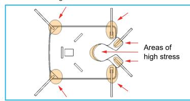
Checks should be carried out to both sides of the sling in the same manner.
