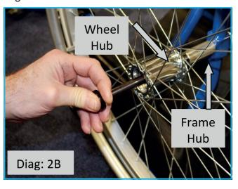
Align the wheel hub with the hub on the frame and push the axle through the frame hub. Diagram 2.
