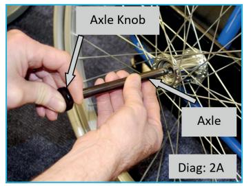
Assemble the wheel axle to the wheel as shown in diagram 2A. Note The axle knob (black) at the end of the axle needs to be pressed in - this will retract the spring locking buttons and allow the axle to pass through the wheel hub.
