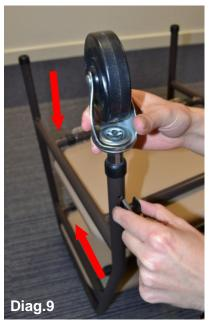
11- Fit the castors to the frame by pushing them into the bottom of the frame, align the holes in the frame with the holes in the castor leg and secure with eclip. See diagram 9, repeat for all four castors, ensuring they are all at the same height. Turn product upright and check it is level and stable.
