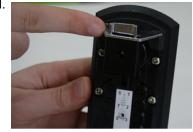
5. Unscrew the small screw that holds the numbered plastic plate in position. Now remove the plate from the facia.
