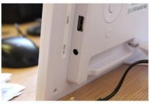
Plug the power cable into the DC IN socket on the side of the frame. Then plug the cable into the mains and switch on at the socket.
