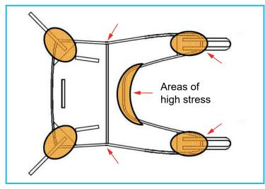
Checks should be carried out to both sides of the sling in the same manner.
