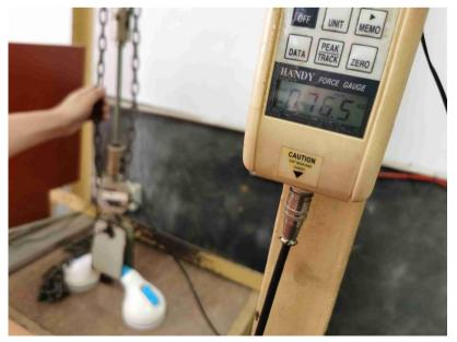
3) When the tensile force reaches 189 lbs / 86 kgs, the suction cup falls off .
