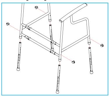
Insert the legs and set to the correct height for the toilet and user, then secure with the 4 x e-clips.
