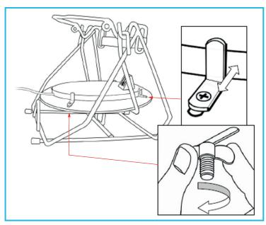
Secure the kettle base onto the tilt plate using the clamps and wing-nuts provided.
