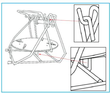
The tilt-plate-stopper must be positioned behind the bar across the base of the frame.
