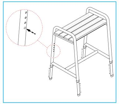
Push and hold the leg button-clips, then slide the legs to the required height until the button-clips click into position in the holes.
