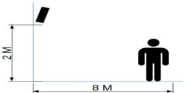
Detection distance of up to 8 Metres with unit mounted at a height of 2 Metres on wall.
