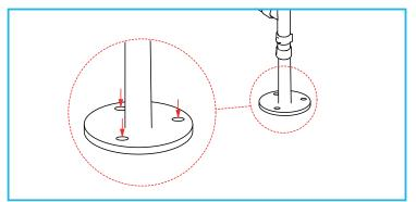
Place the toilet frame in the required location and mark the hole positions to be drilled.
