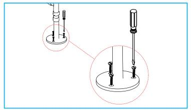
Using an appropriate tool for the chosen fixings, secure the floor fixing kit feet to the floor.
