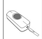
Insert 1 x CR2032 button cell battery, ensuring it is positive (+) side up.
