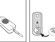
Insert 1 x CR2032 button cell battery, ensuring it is positive (+) side up.
