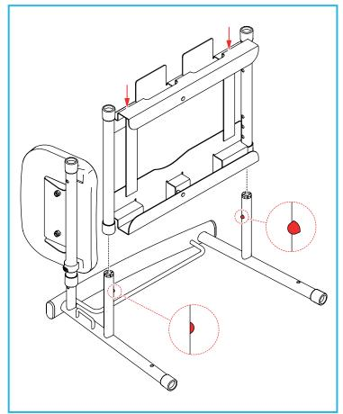
Slot the seat-frame assembly onto the LH sideframe assembly.
