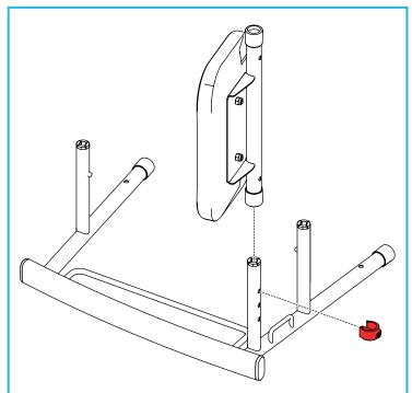
Slot the backrest assembly onto the side-frame assembly (LH) and secure with 1 x E-clip.
