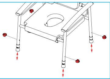
Remove the 4 x E-clips and adjust the legs to the desired height.
