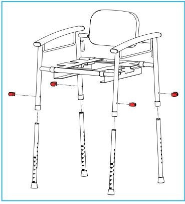
Insert the legs into the side frame assemblies and secure with  $4 \times E$ -clips.
