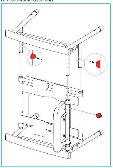
Slot the RH side-frame assembly into the seat/ backrest assemblies.
