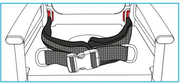
Pull the straps from the front to locate the buckles (B) as shown. Make sure the buckles cannot pull through the seat, by tugging firmly.
