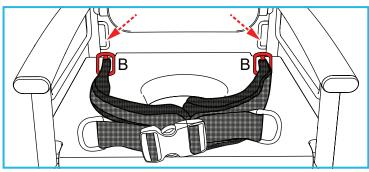
To fit the lap-strap, feed the two rear buckles (B) through the slots in the seat.
