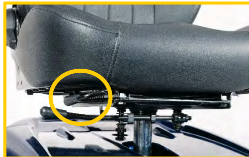
Figure 3 – Pull black handle to adjust the seating position
