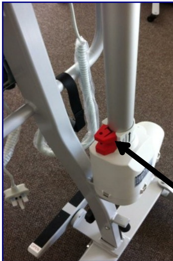
Check 11 Ensure hooks are not damaged and the M10 bolt is secure
