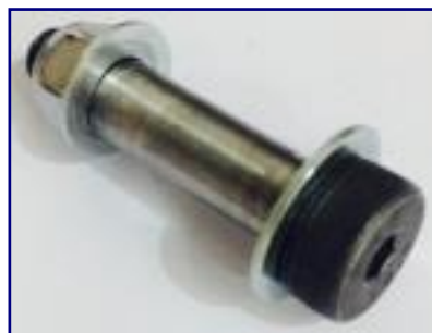
Check 11 Ensure hooks are not damaged and the M10 bolt is secure
