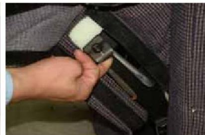
\* Note: To remove the back, pull the spring strips out and up simultaneously.
