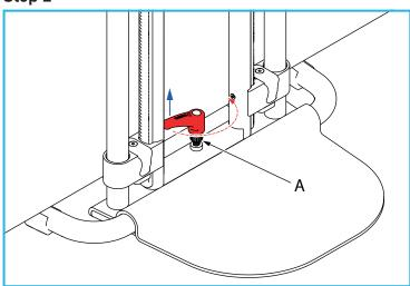
Lift the tightening lever to disengage it from the thread. While holding the lever up, rotate it anti-clockwise by half a turn.
