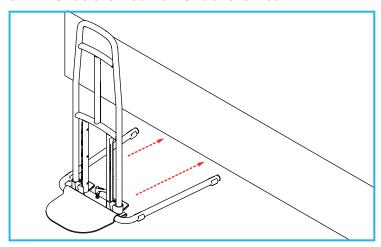
Slide the bed rail under the bed, in an approximate position, until the handrail contacts the bed.
