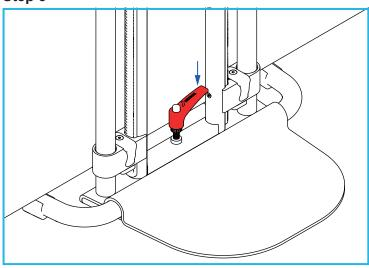
Release the tightening lever, this will re-engage the thread.
