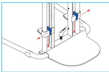
Slide the blue clamp levers outwards to unlock the ratchet clamps. While holding the clamp levers open, slide the ratchet clamps down until they make contact with the base.
