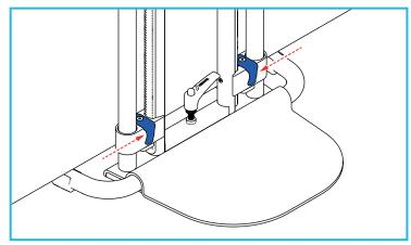
Release the blue ratchet clamp lever to lock the clamps in place.
