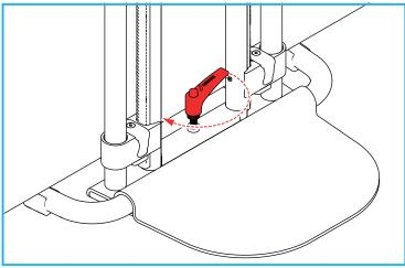
Rotate the tightening lever clockwise by half a turn.
