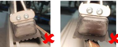
3. The Gripline ends of both sides of the ramp must rest firmly on the level surface.
