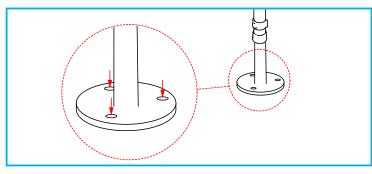
1. Place the toilet frame in the required location and mark the hole positions to be drilled.
