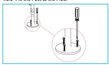
1. Using an appropriate tool for the chosen fixings, secure the floor fixing kit feet to the floor.
