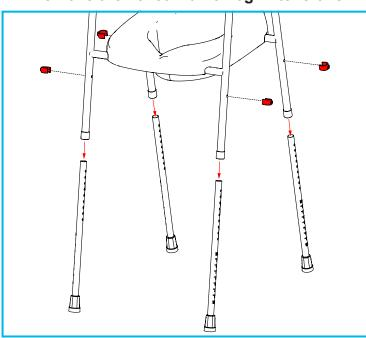
1. Remove the 4 x E-clips, then remove the toilet frame leg extensions.
