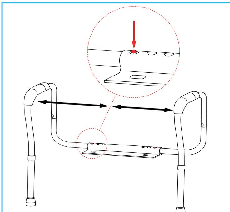
Press and hold the handrail assembly button clip, then slide the handrail to the desired position until the button clip clicks into place.
