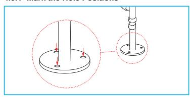
Place the toilet frame in the required location and mark the hole positions to be drilled.
