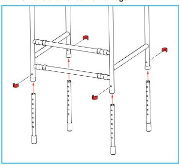
1. Remove the 4 x e-clips, then remove the toilet frame legs.
