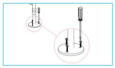
Using an appropriate tool for the chosen fixings, secure the floor fixing kit feet to the floor.
